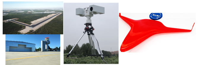
Figure 2: INTA's three contributions to EXAELIA. The selection of a suitable flight test site for project next phases (left) comes with the use of Sistema Portable Óptico de Trayectoria or Optical Portable Trajectory System (SPOT) (center) for on-ground measurements of flight testing demonstrators flights. Hazardous Flight Conditions (HFCs) control laws for said demonstrators is the third leg of INTA's contribution. Up today, several mock-ups have been printed at INTA (right) to identify main stability issues on BWB configurations. Final EXAELIA configuration is yet to be defined as a team effort between several international partners.
