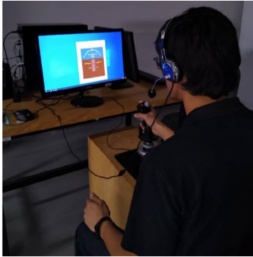
Figure 3: Simulation environment setup, featuring the artificial horizon display (top), joystick control interface (middle), and a pilot performing the simulation task (bottom) [11].
