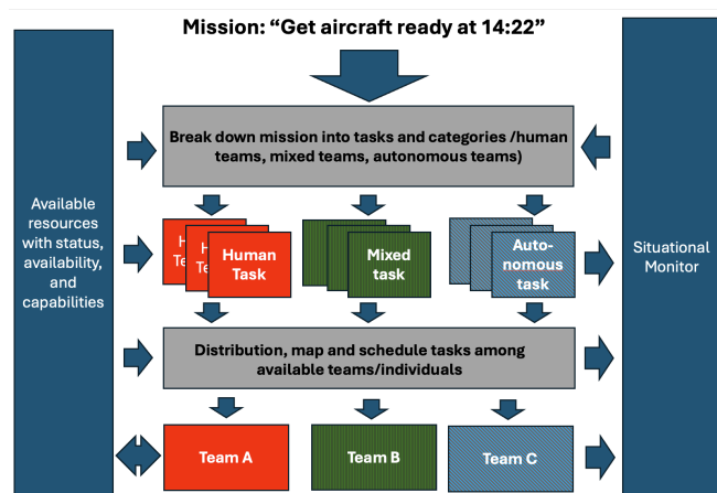
Figure 2: Example of a mission in aviation and how it is broken down into tasks mapped to available resources.
