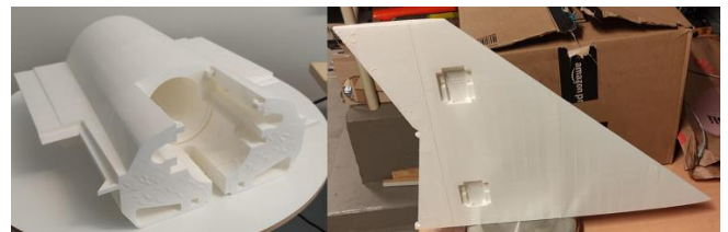
Figure 5: 3D-printed engine section and main wing without control surfaces.
