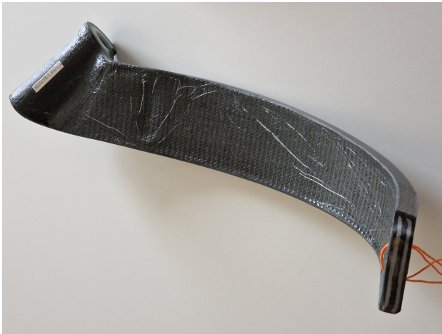
Figure 4: Main Landing gear, "leg".
