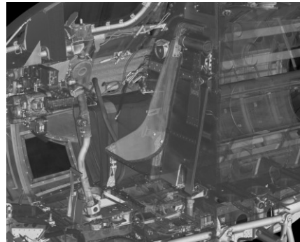
Fig. 1: 3D-CT-rendering of a WWII airplane cockpit (Fraunhofer IIS, EZRT/ Deutsches Museum, CC BY-SA 4.0). 5
