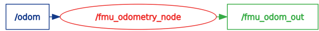
Figure 6. ROS2 node structure for the odometry FMU input subscription to /odom and output publication to /fmu_odom_out .
