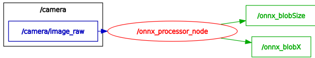
Figure 8. ROS2 node architecture for ONNX integration, illustrating input from the camera feed and output topics for sign detection parameters.
