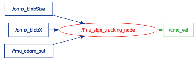
Figure 10. ROS2 node architecture for the SignTrackingLogic FMU, showing input subscriptions from image processing and odometry nodes, and output publication to robot control.
