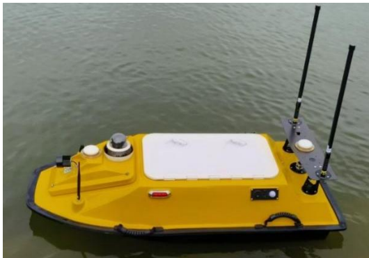
Figure 3. Physical Image of USV130 Unmanned Submarine USV130 is equipped with Ubuntu 20.04 operating system and ROS noetic robot framework, and the underlying motion control adopts PID algorithm. The driving system supports multimodal operation: it can be controlled by the physical remote-control device, the upper computer software and the handle linkage or executed by the autonomous command based on the algorithm. The communication system is equipped with a dedicated base station to achieve stable data transmission with an effective radius of 200 meters.
