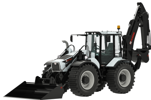
Figure 2. Illustration of an articulated excavator-loader, the Huddig 1370T—an example of a mobile machine capable of both road transportation and load handling, featuring a front loader and a rear excavating unit.
