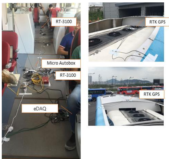
Fig. 10 BRT test equipment setup
