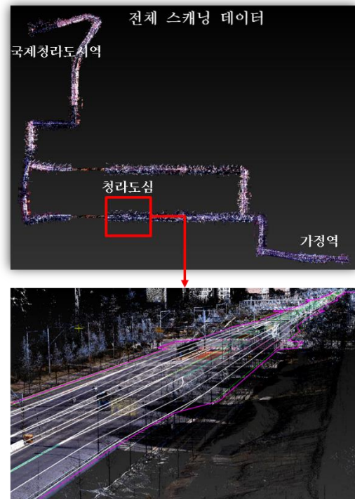
Fig. 2 Scanned las data of BRT route
