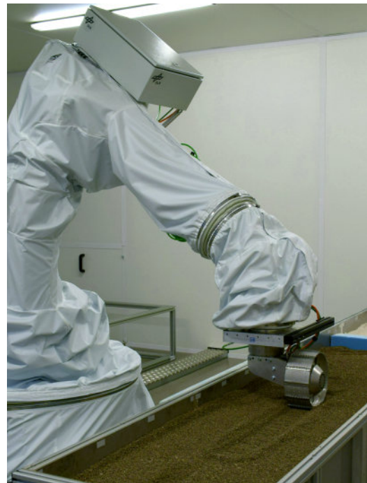
Figure 6. Side view of the TROLL showing the robot, force torque sensor, drive unit with wheel and a soil bin filled with lava sand.
