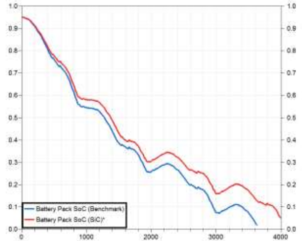
Figure 10 Charging state (SOC) of the EV traction battery when adopting the driving profile “Artemis Motorway”.
