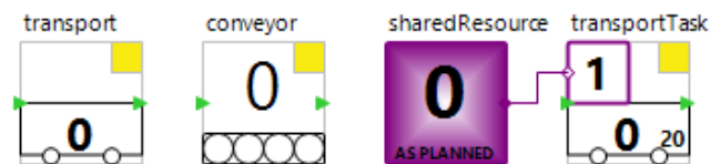
Figure 3. Transport devices of the process simulation library. From left to right: transport, conveyor, and shared resource with transport task.
