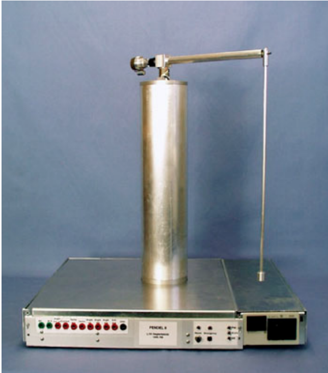
Figure 3. Photograph of Furuta pendulum.
