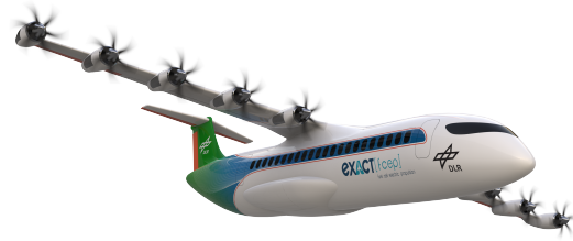
Figure 1. LH2 driven Fuel Cell Aircraft from EXACT project.
