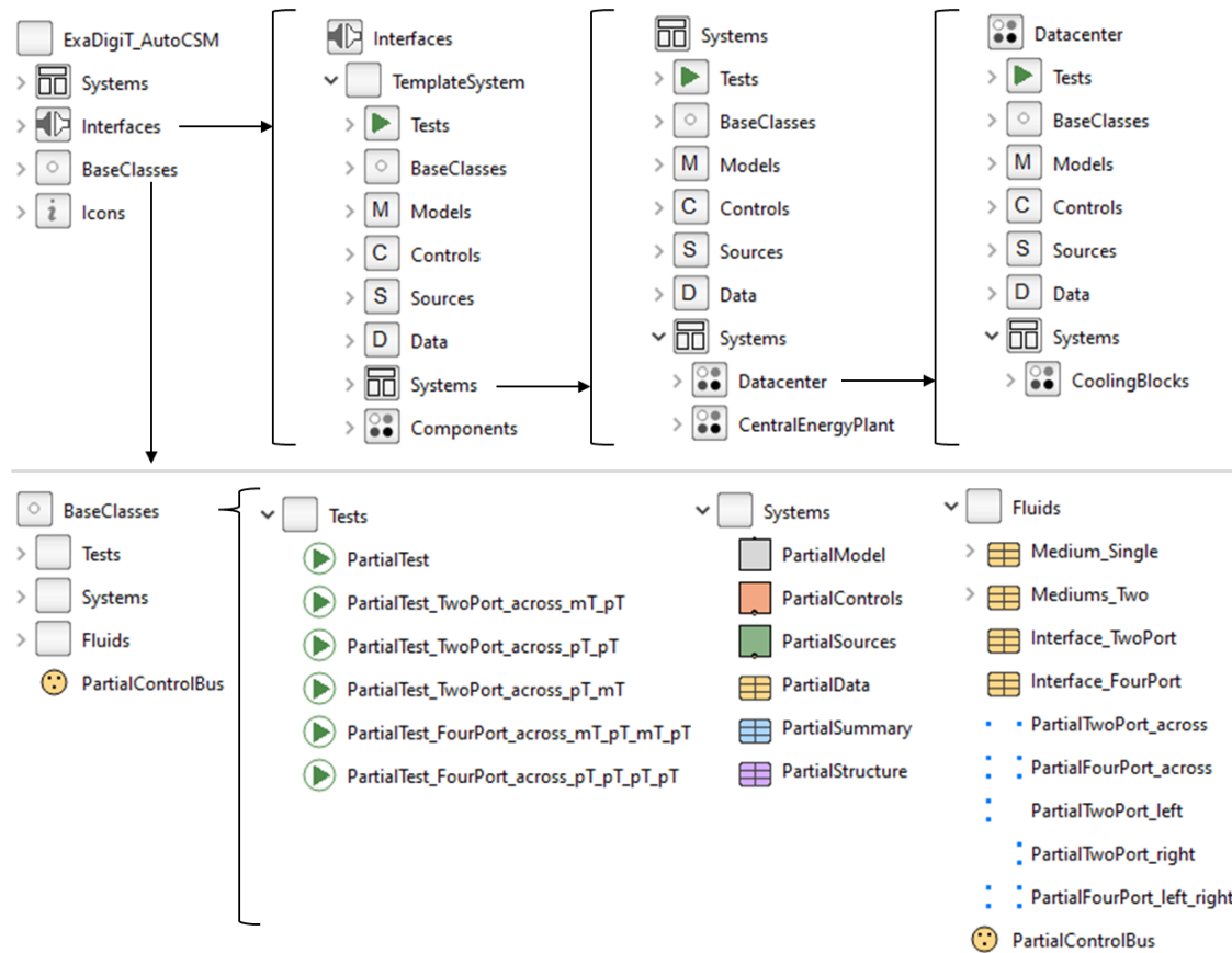
Figure 4. ExaDigiT Modelica template library. All systems use a common TemplateSystem that is then modified for the specific system. The TemplateSystem relies on replaceable components built on the (BaseClasses) models.
