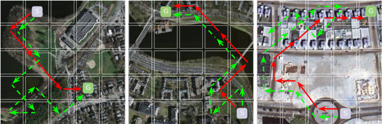
Fig. 2. Examples of AiRLoc (red) and Priv local (dashed green) on the test set of Masa (left, middle) and Dubai (right). Left: AiRLoc takes the same first two actions as Priv local and then takes the shortest path to the goal ('G'). Priv local also reaches the goal. Middle: AiRLoc first deviates from Priv local and then follows the same path. AiRLoc reaches the goal faster. Right: AiRLoc follows the same path as Priv local until it is adjacent to the goal and then moves into the goal, while Priv local fails.
