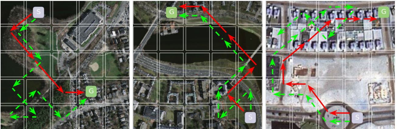
Fig. 2. Examples of AiRLoc (red) and Priv local (dashed green) on the test set of Masa (left, middle) and Dubai (right). Left: AiRLoc takes the same first two actions as Priv local and then takes the shortest path to the goal ('G'). Priv local also reaches the goal. Middle: AiRLoc first deviates from Priv local and then follows the goal faster. AiRLoc reaches the goal faster. Right: AiRLoc follows the same path as Priv local until it is adjacent to the goal and then moves into the goal, while Priv local fails.
