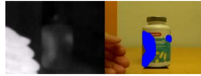
Figure 4. Example of a simplified approach for extracting heat traces and not humans via thresholds, morphology, and a basic shape model for touching: (a) thermal image, (b) RGB image with heat traces drawn by the algorithm
