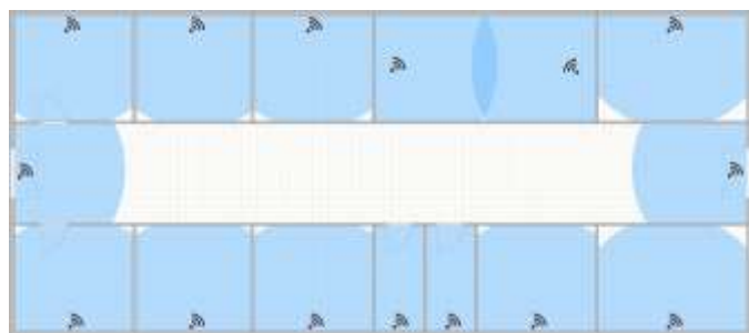
Figure 1 - An example of beacon network floor coverage
