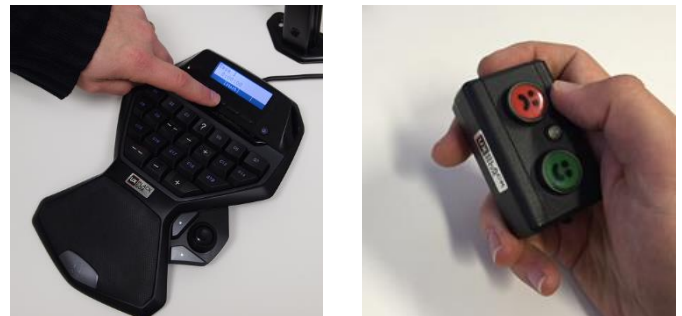
Figure 2 - Left: A commercial game control pad is used as the moderator pad, which is configured to keep track of test session status on display and to provide buttons for making marks during test sessions.
