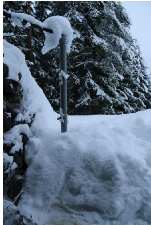
Figure 1: The prototype, covered by about 70 cm with snow. The two upper capacitance sensors can be seen as the two black objects pointing to the left of the pipe.
