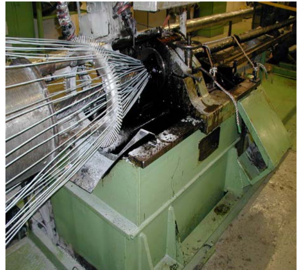
Figure 2: Wires being coated with bitumen
