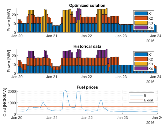
Figure 5. Top: Proposed solution from algorithm for the period 20-24 Jan 2016. Mid: Actual power output from historical data for the same period. Bottom: Actual fuel prices from the same period.
