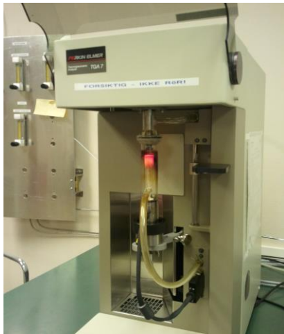
Figure 3: Experimental set up of TGA.
