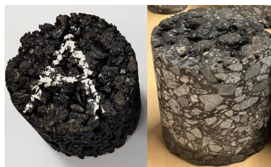
Figure 1: The porous (left) and regular asphalt (right) samples considered in this work.
