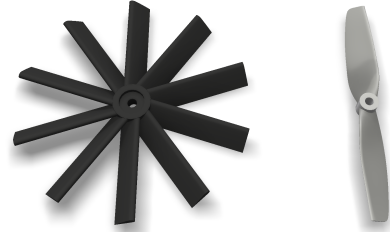
Figure 2. 3D-printed low-efficiency (left) and high-efficiency (right) propellers (left)
