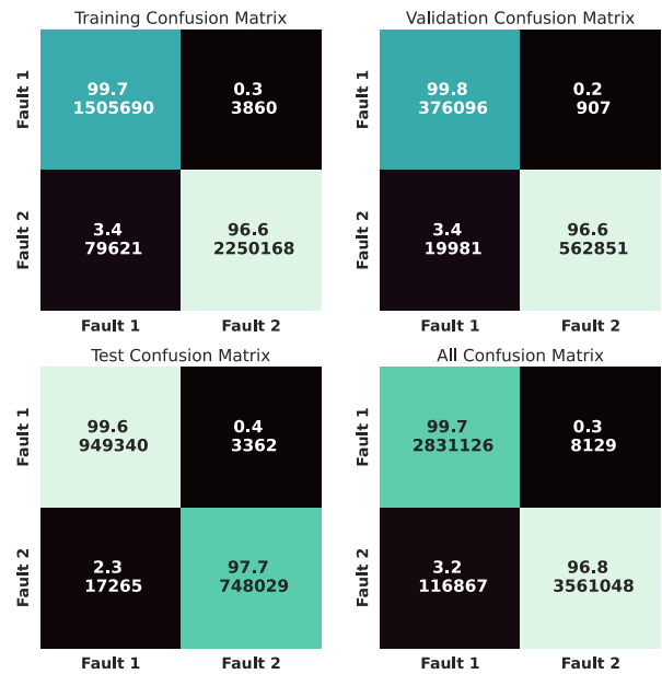
Fig. A2. CNN confusion matrix for training, validation, testing, and total dataset
