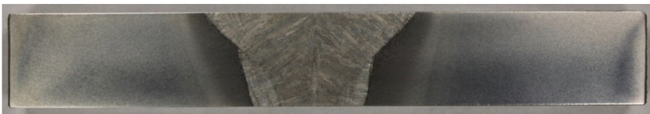
Fig. 1. Specimen for the physical simulation of the heat-affected zones with the original weld metal in the middle.
