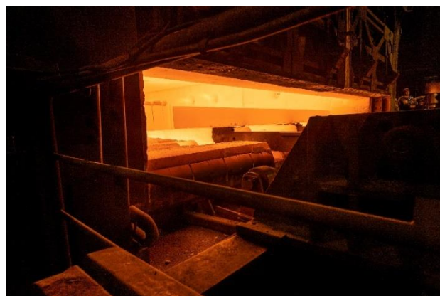
Fig. 5. Bloom with thermoelements being discharged from the furnace.
